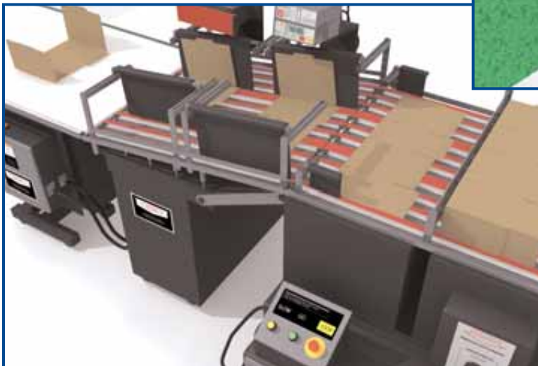
Its combined characteristics of high friction and abrasion resistance make the seamless Thermoplastic Rubber backing ideal for box folding applications.
