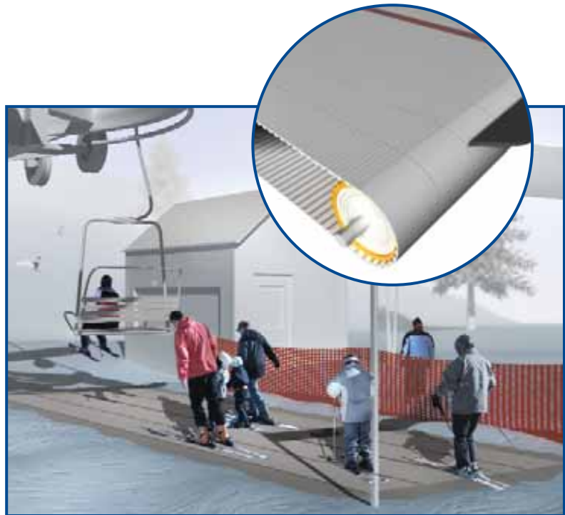
Four 450 mm wide, timing belts accelerate skiers for faster loading of detachable chair lifts. Timing belts ensure uniform speed of each skier.
